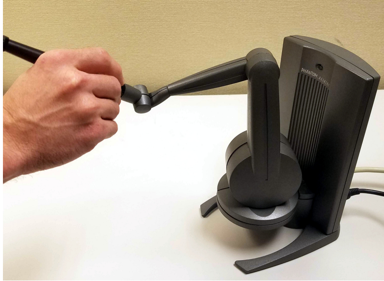
Figure 3.1: Sensable Inc's PHANToM Desktop, a force feedback device for haptic applications
