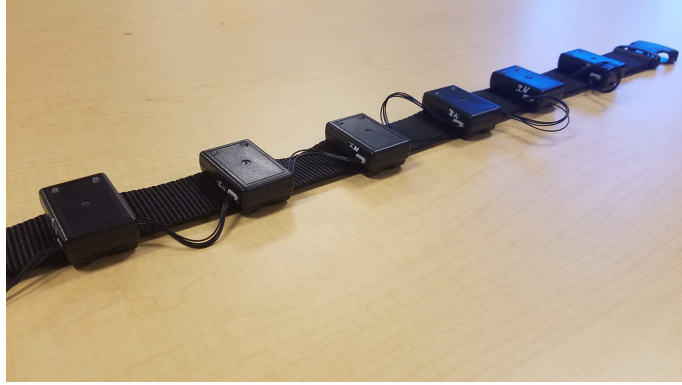
Figure 3.3: Haptic Belt developed at the CUbiC Lab at Arizona State University Rosenthal et al. (2011). The belt was designed to be modular and can be extended to fit more or fewer tactors connected in series. The location of the tactors can also be modified by simply sliding them along the belt.
