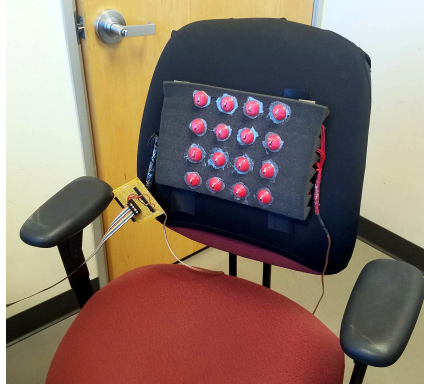
Figure 3.6: The Low Resolution Haptic Display, a 4x4 array of vibration motors mounted vertically on acoustic foam for compliance and damping Fakhri et al. (2019)
